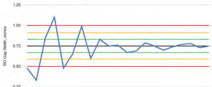
Control Chart - Window RO Gaps
